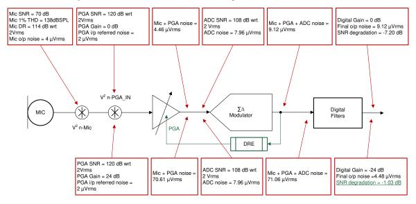
Figure 5-1. DRE Block Diagram
