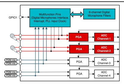
Figure 6-4. Combination Microphones System Block Diagram
