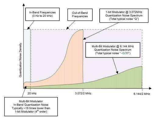
Figure 4-1. Quantization Noise Density
