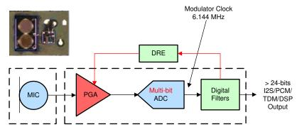
Figure 3-2. Analog Microphone with ADC for Multi-bit Output
