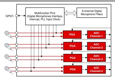
Figure 6-2. Analog Microphones System Block Diagram
