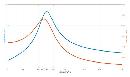
Figure 5. Impedance and Excursion Simulation Result with Matlab Based on Speaker Model
