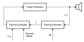
Figure 11. Thermal Protection in Smart Amp Algorithm
