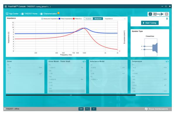
Figure 6. Impedance and Excursion Characterization Result with PPC3 and LB2
