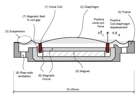
Figure 2. Typical Speaker Structure
