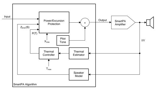
Figure 7. Smart amp Algorithm
