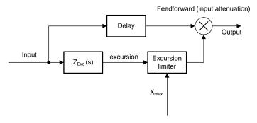
Figure 8. Excursion Protection System in Smart Amp Algorithm
