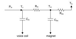
Figure 12. Typical Thermal Model of Speaker
