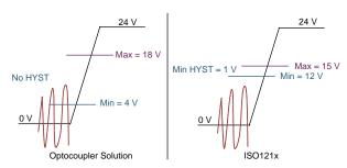
Figure 3. ISO121x Based Receivers Have Higher Noise Margin to the High and Low Levels
