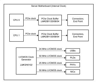
Figure 3. Example server motherboard internal clock architecture.
