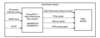
Figure 13. Simplified spine or fabric switch clock architecture.
