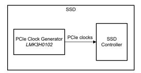
Figure 9. Example PCIe SSD clock architecture.
