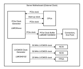
**Figure 4.** Example server motherboard external clock architecture.
