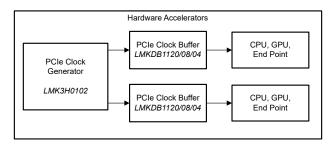
Figure 8. Example hardware accelerator clock architecture.
