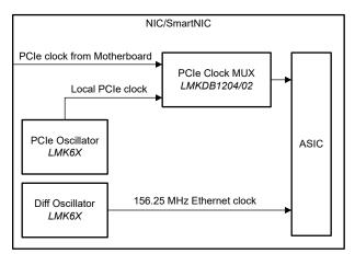
Figure 7. Example NIC and SmartNIC clock architecture.
