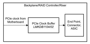
Figure 6. Example PCIe add-in cards clock architecture.
