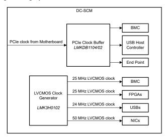
Figure 5. Example DC-SCM clock architecture.
