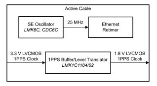
Figure 11. Example active cable clock architecture.
