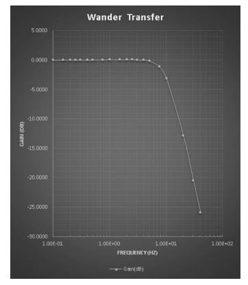
Figure 3-2. Wander Transfer EEC Option 1 With Max DPLL Bandwidth of 10 Hz
