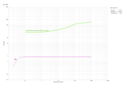
Figure 2-3. Wander Generation MTIE Option 1, G.8262 EEC Option 1 Results, Tested at Temperature of 85°C With DPLL Bandwidth of 10 Hz
