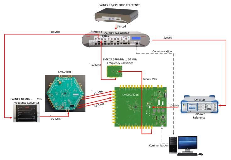
Figure 6-1. Test Setup for Phase Transient Generation
