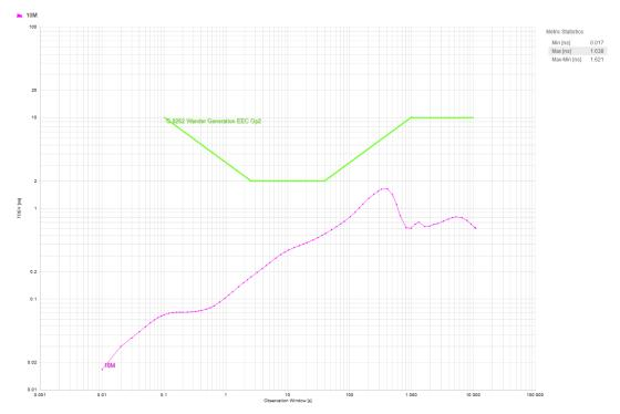
Figure 2-6. Wander Generation TDEV G.8262 EEC Option 2 Results, Tested at Constant Room Temperature With DPLL Bandwidth of 0.1 Hz
