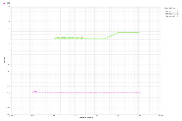
Figure 2-4. Wander Generation TDEV G.8262 EEC Option 1 Results, Tested at Constant Room Temperature With DPLL Bandwidth of 10 Hz
