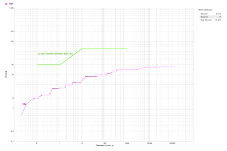
Figure 2-5. Wander Generation MTIE ITU-T G.8262 EEC Option 2 Results, Tested at Constant Room Temperature With DPLL Bandwidth of 0.1 Hz
