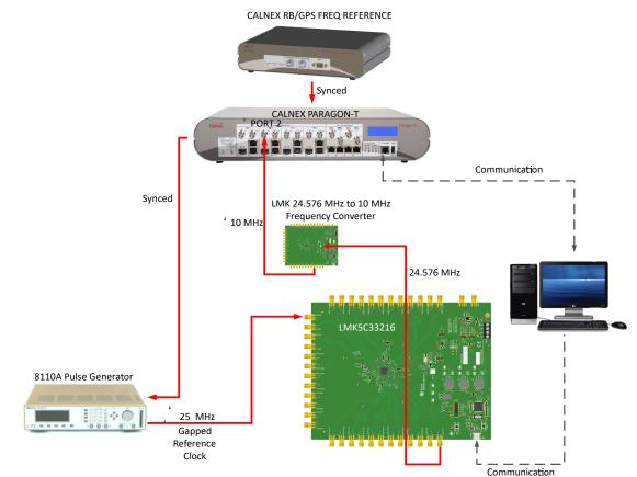
Figure 6-4. Test Setup for Phase Transient Generation With Signal Interruption
