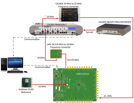
Figure 3-1. Test Setup for Wander Transfer
