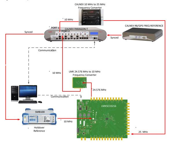
Figure 4-1. Test Setup for Wander Tolerance
