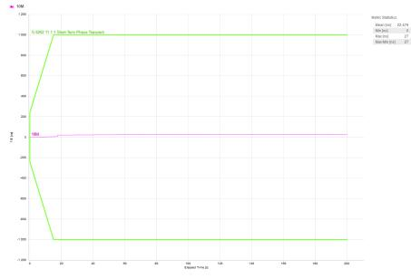
Figure 6-2. Short-Term Phase Transient Result
