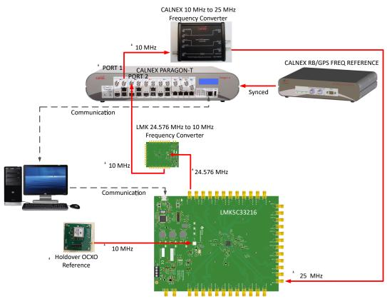
Figure 2-1. Test Setup for Wander Generation
