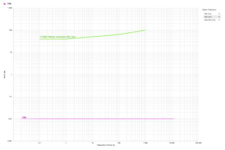
Figure 2-2. Wander Generation MTIE Option 1, G.8262 EEC Option 1 Results, Tested at Constant Room Temperature With DPLL Bandwidth of 10 Hz
