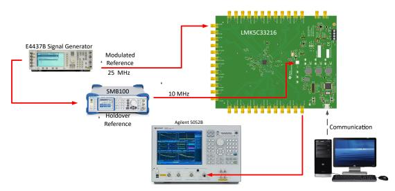
Figure 5-1. Test Setup for Jitter Tolerance
