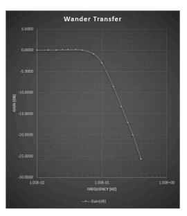
Figure 3-3. Wander Transfer EEC Option 2 With Max DPLL Bandwidth of 0.1 Hz
