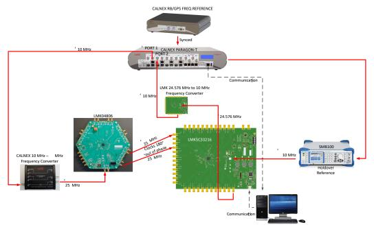
Figure 6-6. Test Setup for Phase Discontinuity
