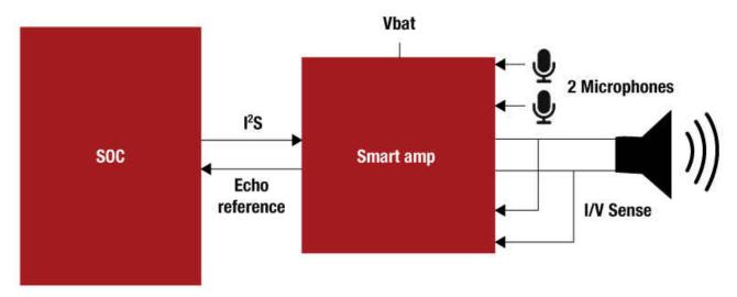
Figure 2. Smart Amps Integrate Most Components of a Two-way Audio System in a Single Package
