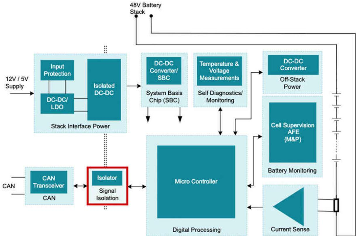
**Figure 2. 48-V BMS block diagram**
