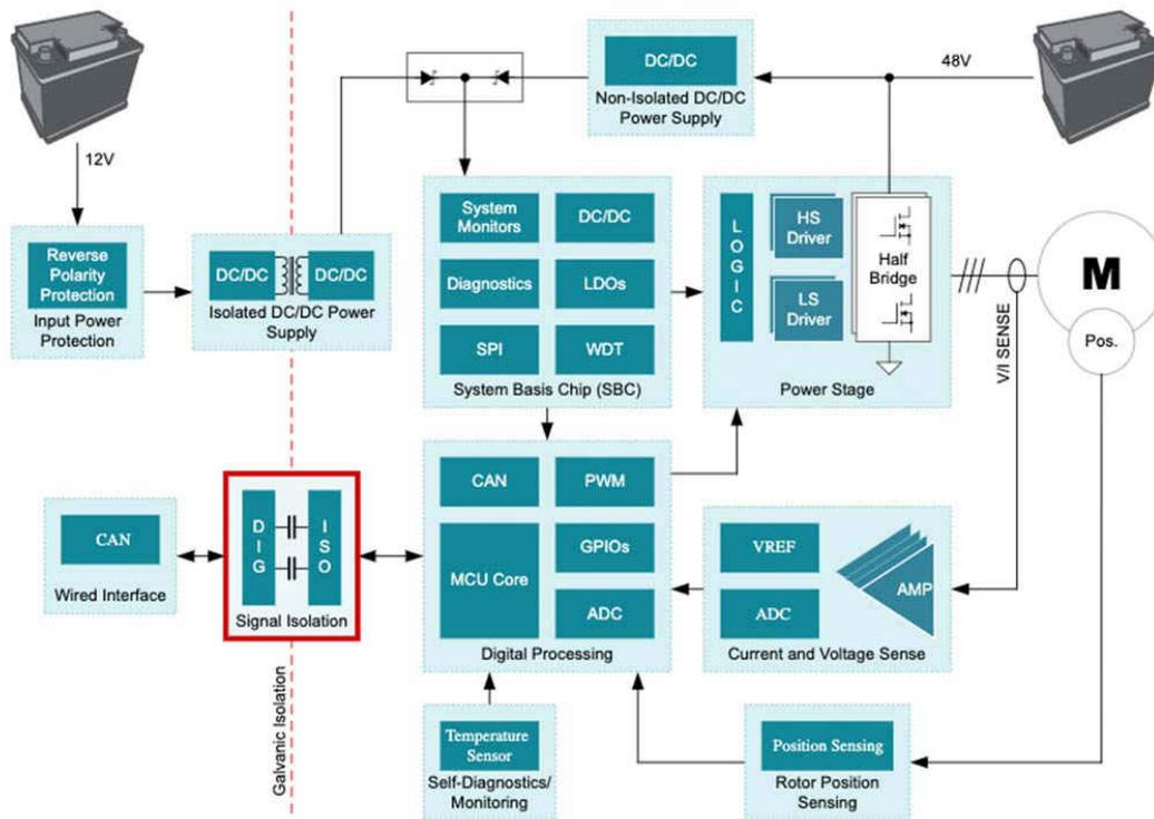
Figure 1. Starter/generator subsystem in a 48-V HEV
