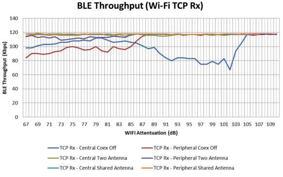
Figure 4-3. BLE Throughput During Wi-Fi<sup>®</sup> TCP Rx
