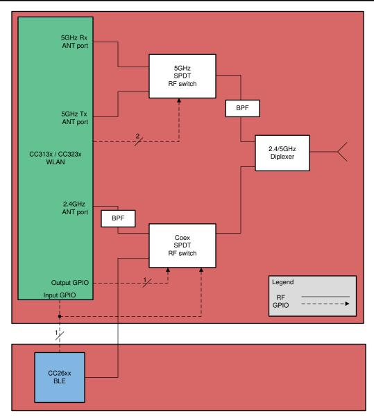
Figure 2-2. BLE Coexistence Block Diagram
