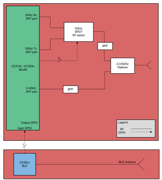
Figure 2-3. BLE Coexistence Block Diagram, Dual Antenna
