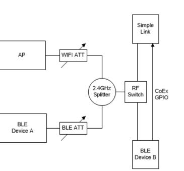
Figure 4-1. Shared Antenna Test Setup
