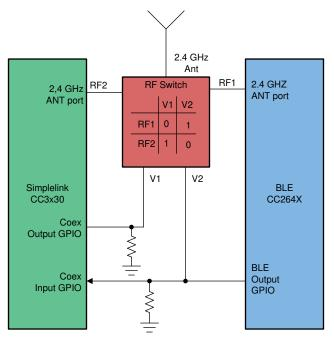
Figure 1-1. System Block Diagram
